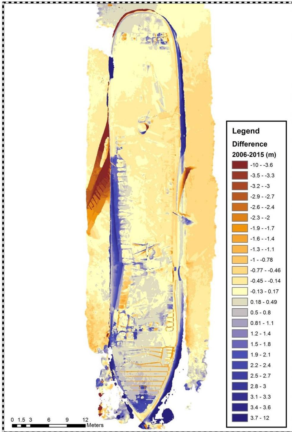
Figure 6: Change map of the Wisconsin, with amounts of change indicated: blue are areas of loss or collapse, and red are areas of gain (Jordan Mertes, Jason Gulley, Michigan Technological University)
